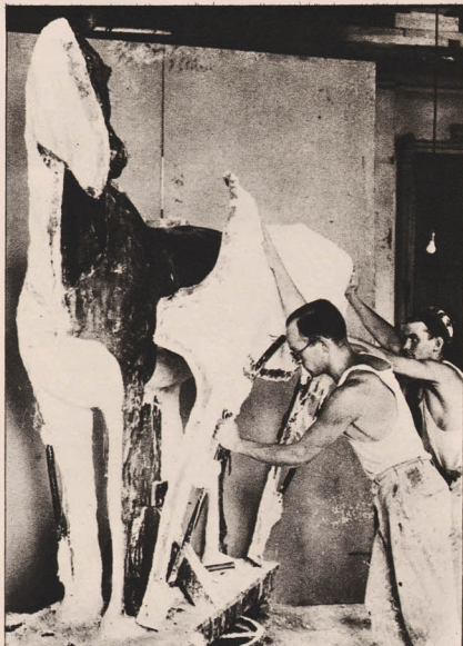
4 Off Comes the Mold. The section being removed weighs 270 pounds. It requires the steel brace for support and the strength of two men for handling. In this mold, a new figure of Phar Lap is built up of roofing paper, burlap and shellac. The work was done by the Jonas brothers in Mount Vernon, N. Y.
